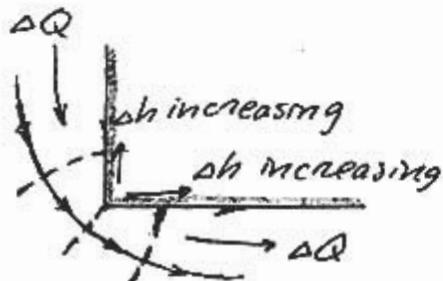
Velocity at corner pointing into flow is high and decreases away from corner
