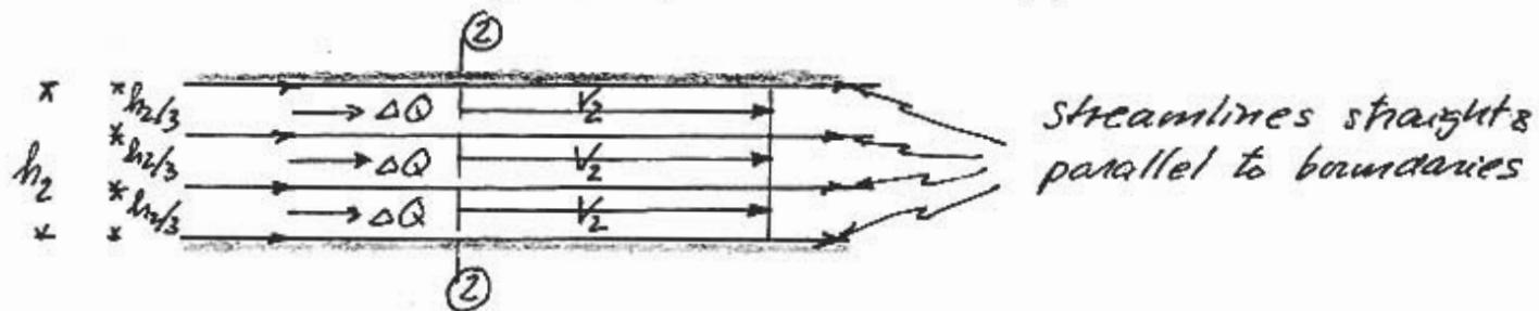
$$Q = h_2 V_2 ; \text{ 3 streamtubes are connected to the 3 streamtubes we had at ①, so each carries a discharge } \Delta Q$$
