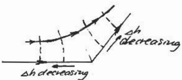
Velocity at corner pointing away from flow is low and increases away from corner.
