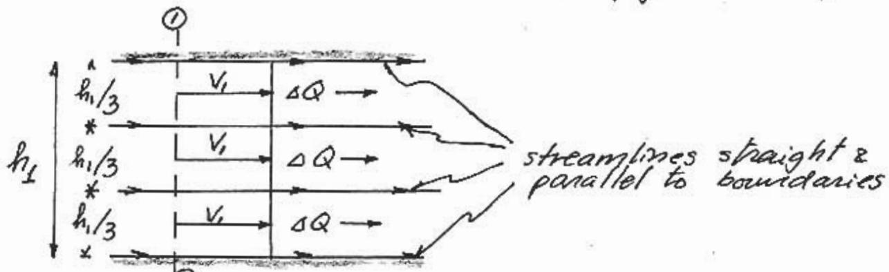
$$Q = h_1 V_1 ; \text{ 3 streamtubes formed by 4 streamlines: } \Delta Q = V_1 \Delta h_1 = V_1 h_1/3 = Q/3$$
