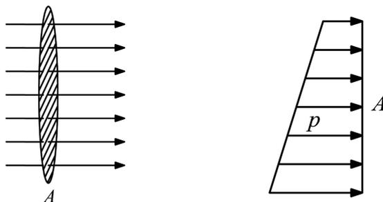
Figure 1: Straight and parallel streamlines passing through the flow area (left); linearly varying pressure (right).
