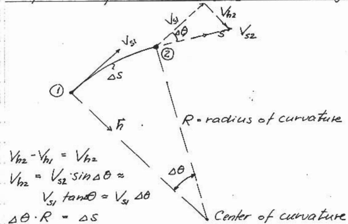
$$\text{So : } \frac{V_{h2} - V_{h1}}{\Delta s} = \frac{\partial V_h}{\partial s} = \frac{V_{h2}}{\Delta s} = \frac{V_{s1} \Delta\theta}{R \Delta\theta} = \frac{V_s}{R}$$
