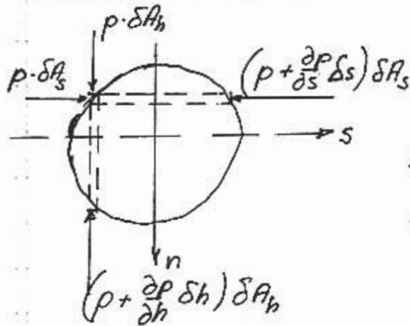
$$\text{Net force: } - \frac{\partial P}{\partial s} \frac{\delta s \delta A_s}{\text{volume of cylinder}} \text{ in } \vec{s}$$
