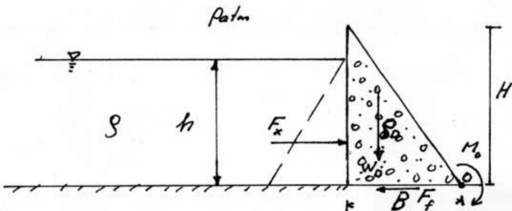
From 2-D hydrostatics we have (per unit length into paper) :
