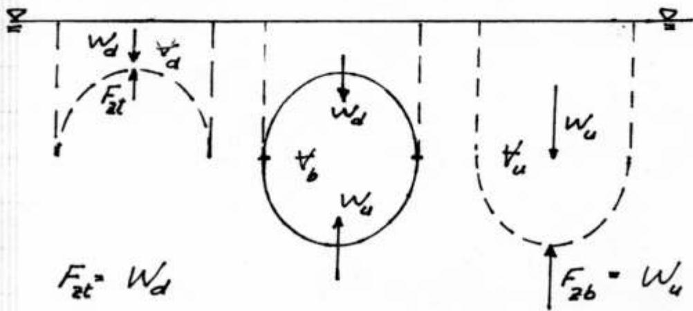
$$\text{Net force on submerged body} = W_u - W_d = \rho g (t_u - t_d) = \rho g t_b =$$
