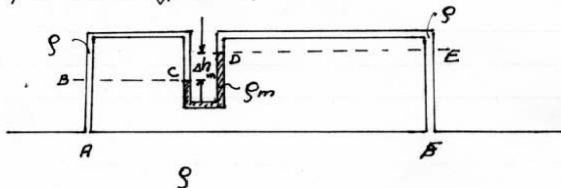
The manometer is connected to the fluid (of density  $\rho$ ) through pressure taps at A and F. The manometer fluid has a density  $\rho_m$  ( $> \rho$ ) and is located in a U-tube. The manometer reading is the difference between the manometer fluid elevations in the two legs of the U-tube,  $\Delta h_m$ .
