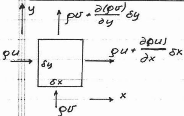
We consider a fixed representative elementary volume (REV),  $\delta t = \delta x \delta y$ , and limit ourselves to two-dimensions (unit length into paper).
