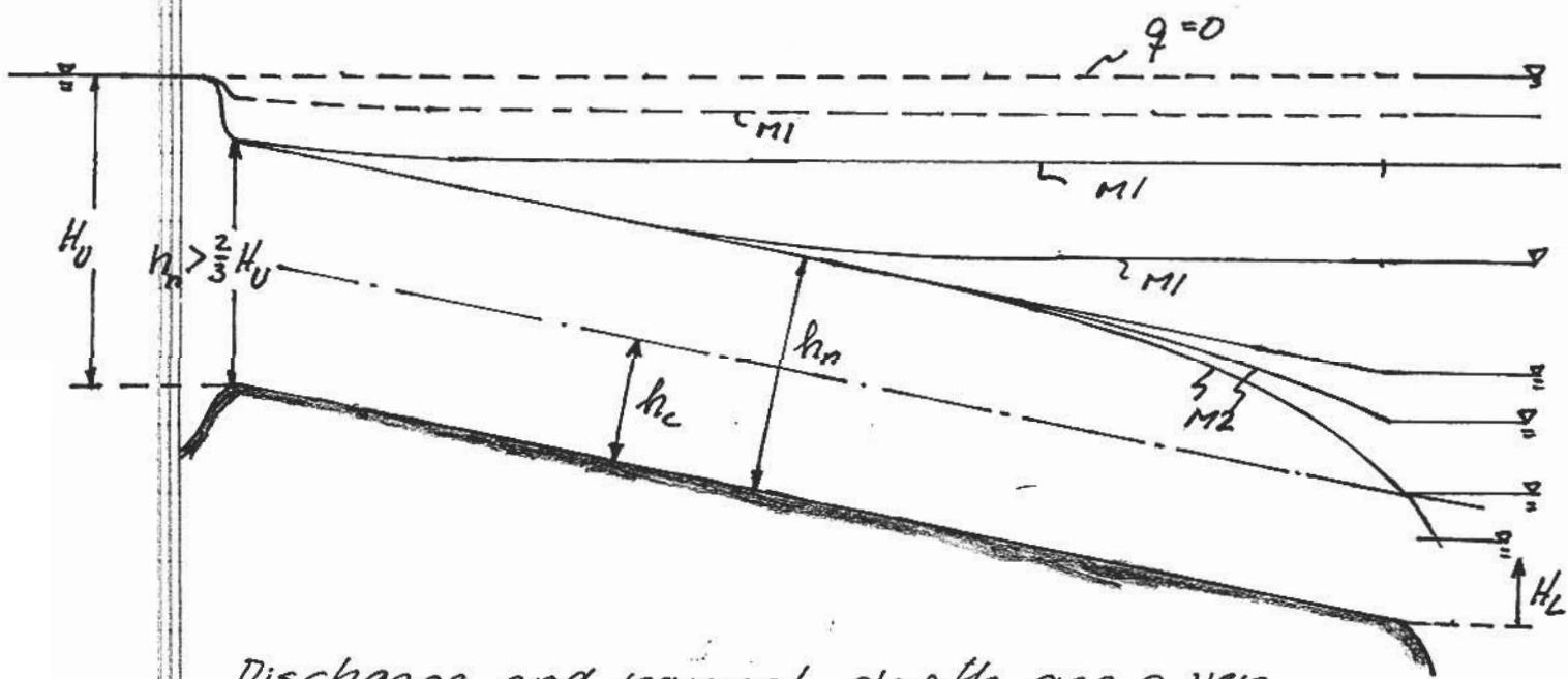
Discharge and normal depth are given by (7) and (8), and  $h_n$  is hit immediately at start of channel and is maintained until influenced by conditions imposed by the
