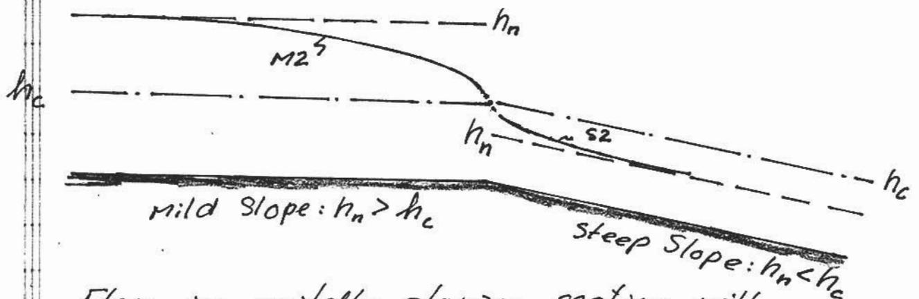
Flow in mildly sloping section will be drawn down to  $h_c$  at the change in slope. Upon entering the steep channel it starts at  $h_c$  and proceeds toward  $h_n$  through a  $S2$ -profile. If the  $M2$ -profile did not hit  $h_c$  at entrance to the steep channel the flow would follow an  $S1$ -profile which would be impossible in the absence of a downstream control.
