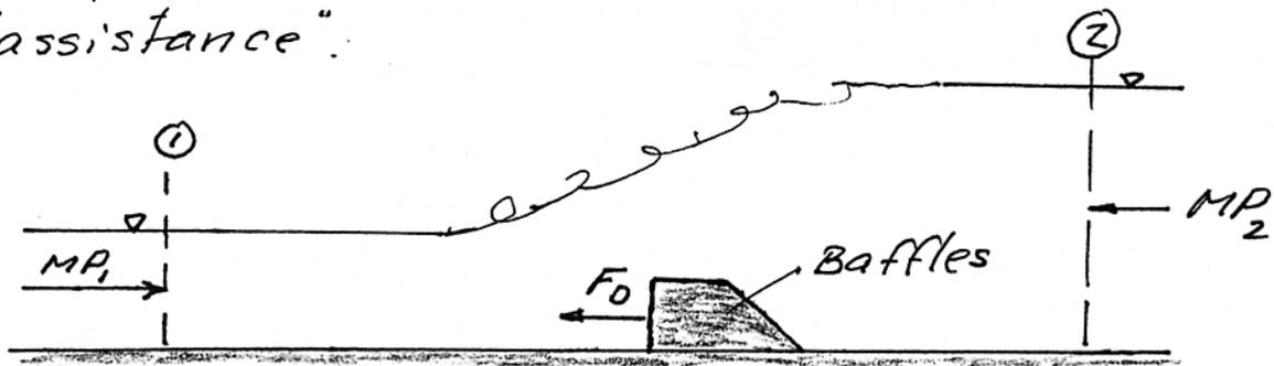
An example of this assistance is baffles, i.e. flow obstructions that produce a drag force on the fluid, that helps to achieve the necessary force equilibrium for the jump:
