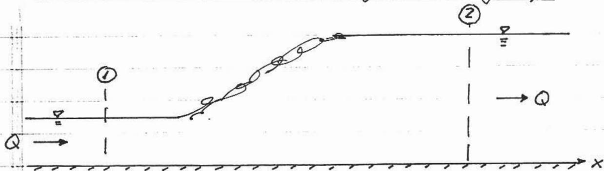
$$MP_1 + \text{Gravity in } x = MP_2 + \text{Friction force from bottom} + \text{Other Forces in } x$$
