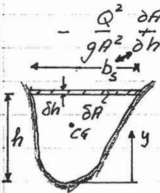
$$- \frac{Q^2}{gA^2} \frac{\partial A}{\partial h} + A + h \left( \frac{\partial A}{\partial h} \right) - \frac{\partial(y_{CG} A)}{\partial h}$$
