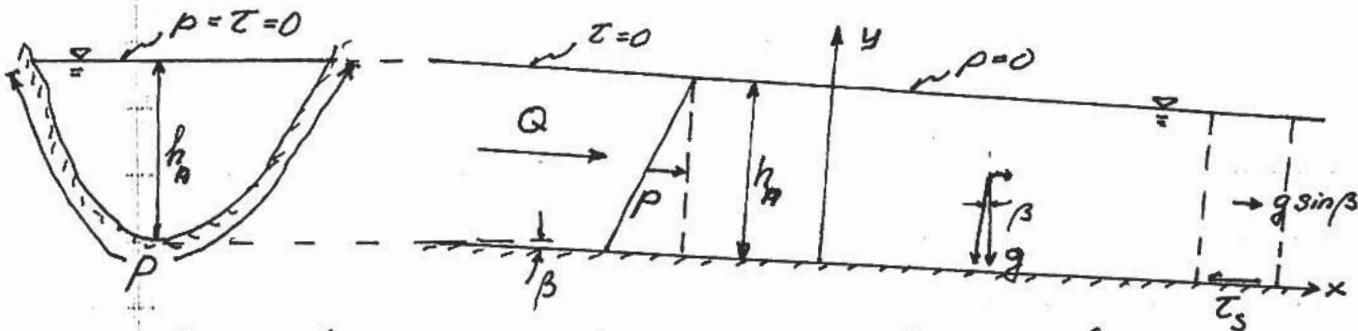
Prismatic channel - cross-section  $\neq f(x)$
