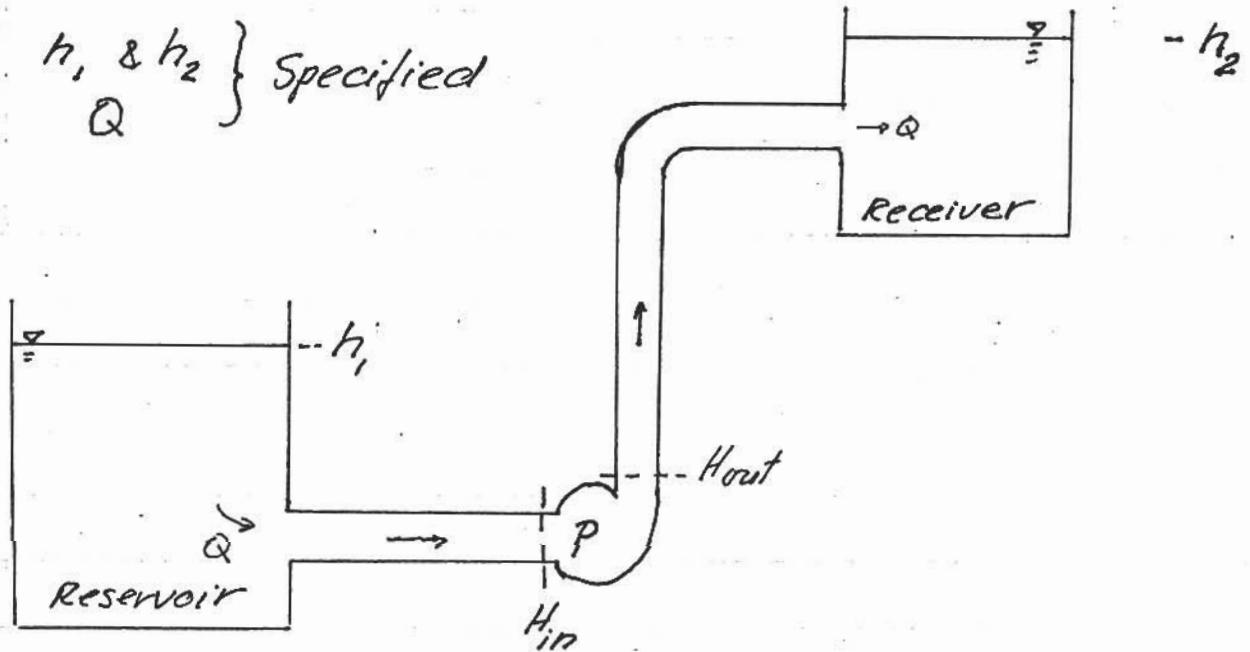
Determination of Pump Head,  $H_p = H_{out} - H_{in}$
