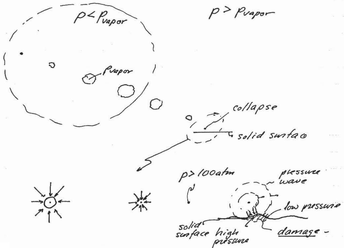
Cavitation must not occur anywhere in Hydraulic Structures and Machinery. To check and make sure that cavitations will not occur we need to determine the pressure (its lowest value) in the system and compare it with the liquid's vapor pressure.
