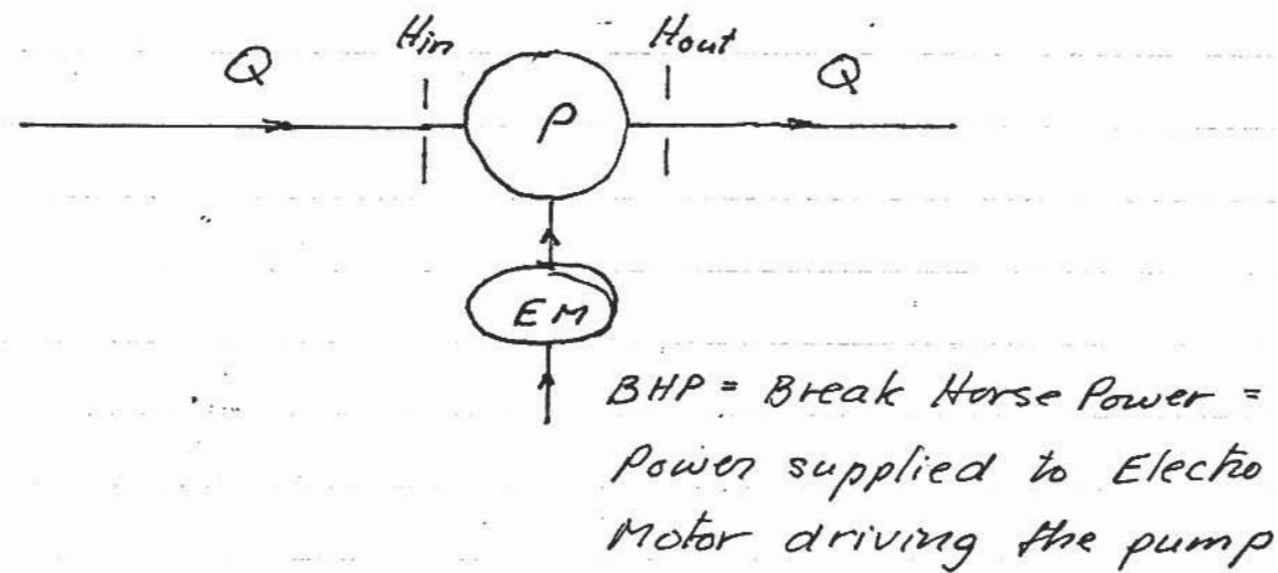
Rate of Mechanical Energy supplied by the Pump to the Flow =  $E_{out} - E_{in} = \rho g Q [H_{out} - H_{in}] = \underline{\rho g Q H_p} = \dot{E}_p$
