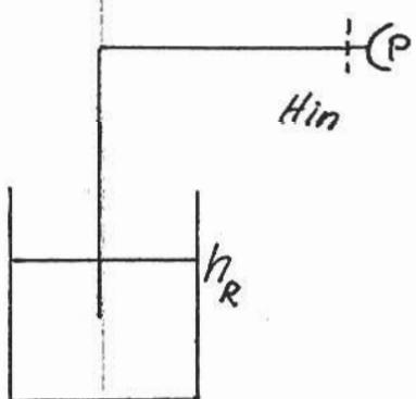
$$H_{in} = \frac{V_{in}^2}{2g} + \frac{P_{Cg,in}}{\rho g} + Z_{Cg,in} = h_R - \Delta H_{rop}$$
