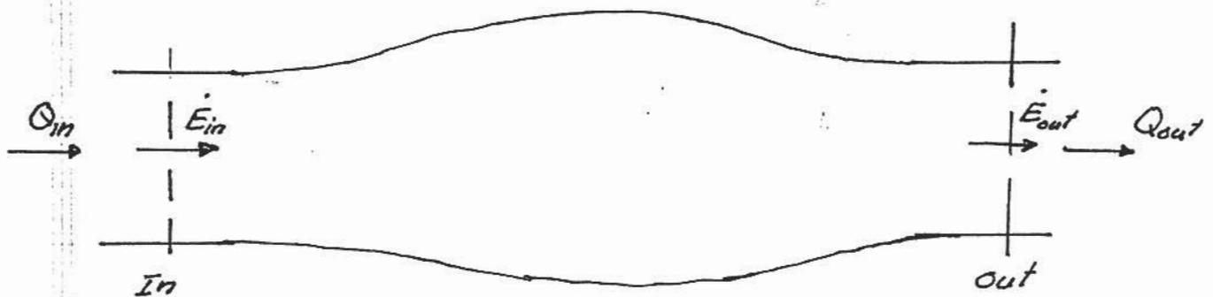
$\dot{E}$  = flow rate of mechanical energy across flow area  $A$  where flow is well behaved =  $\rho g Q H$
