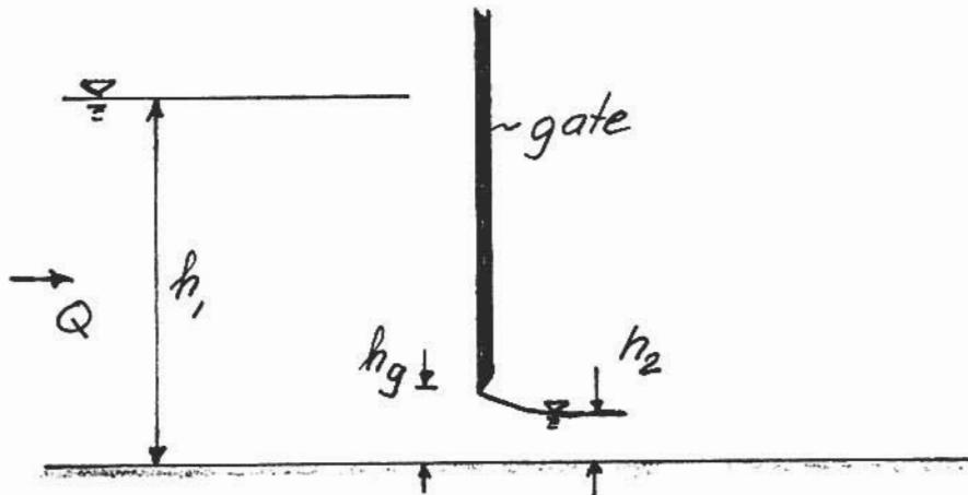
A discharge of  $Q = 100 \text{ m}^3/\text{s}$  passes under a vertical gate located in a rectangular channel of width  $b = 20\text{m}$ . The depth of flow a short distance after passing under the gate is  $h_2 = 0.60\text{m}$  (see sketch).
