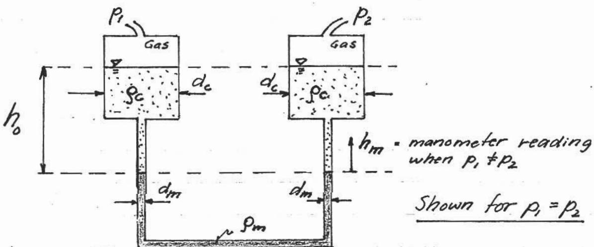
When  $p_1 \neq p_2$  and the manometer reading  $h_m \neq 0$ , say  $h_m > 0$ , then the rise of manometer fluid in right leg forces chamber fluid up into right chamber. Also, if manometer fluid rises in right leg by  $h_m$ , it drops in left leg by  $h_m$  and the level in left chamber drops.
