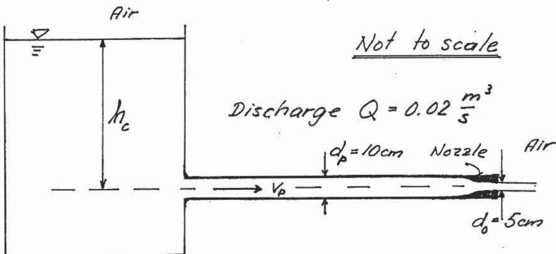
The sketch above shows a horizontal pipe of diameter  $d_p = 10\text{ cm}$ , carrying a discharge  $Q = 0.02 \text{ m}^3/\text{s}$  of water,  $\rho = 1000 \text{ kg/m}^3$ . The discharge is supplied from a very large container in which the water level is a vertical distance  $h_c$  above the pipe elevation. The pipe discharges into the atmosphere through a nozzle with a circular outflow of diameter  $d_o = 5\text{ cm}$ .
