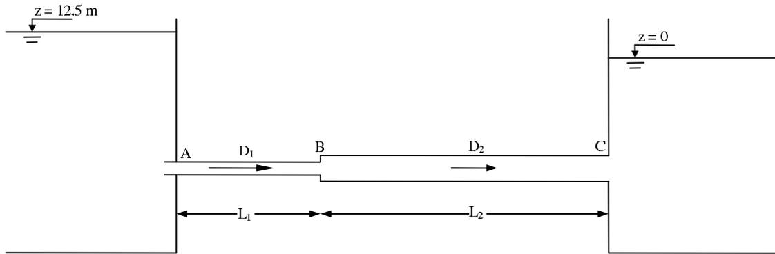
Figure 3: Pipes connecting two reservoirs in Problem 3.
