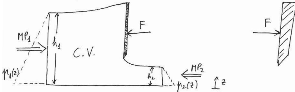
$$MP_1 = (\rho g h_1 + \rho V_1^2) h_1 = \left( \frac{\rho g h_1}{2} + \rho V_1^2 \right) h_1 = \left( \frac{9800 \cdot 3}{2} + 1000 \cdot 1.421^2 \right) \cdot 3 =$$
