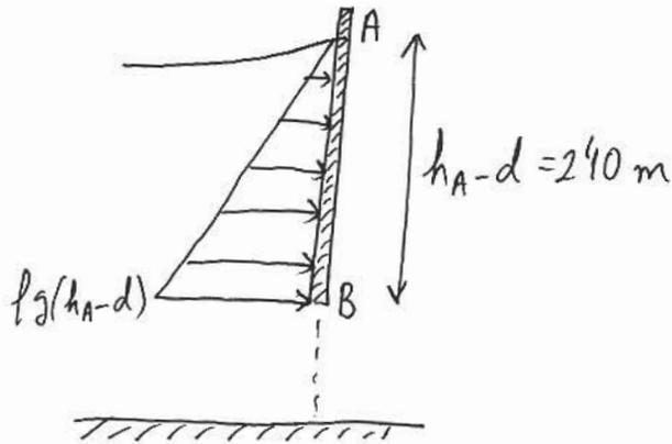
$$\begin{aligned} \underline{F} &= \text{area of the triangle of pressure} = \frac{1}{2} \rho g (h_A - d)^2 \\ &= \frac{9800}{2} \cdot 240^2 = \underline{\underline{21609 \text{ N/m}}} \end{aligned}$$
