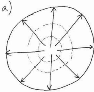
For reasons of angular symmetry, the flow must be purely in the radial direction, i.e., streamlines are straight lines in the radial direction.
