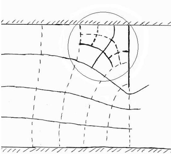
This is an example of a reasonably good flownet. I have subdivided the upper-right weirdo (the one inside the circle) twice. First, I introduced a new streamline AND a new equipotential line (both are drawn as solid lines) to get four sub-weirdos that look reasonably square. Again, I subdivided the two upper sub-weirdos (now I used dashed lines) and get sub-sub-weirdos that are again reasonably square. Therefore, I conclude that the flownet looks right.
