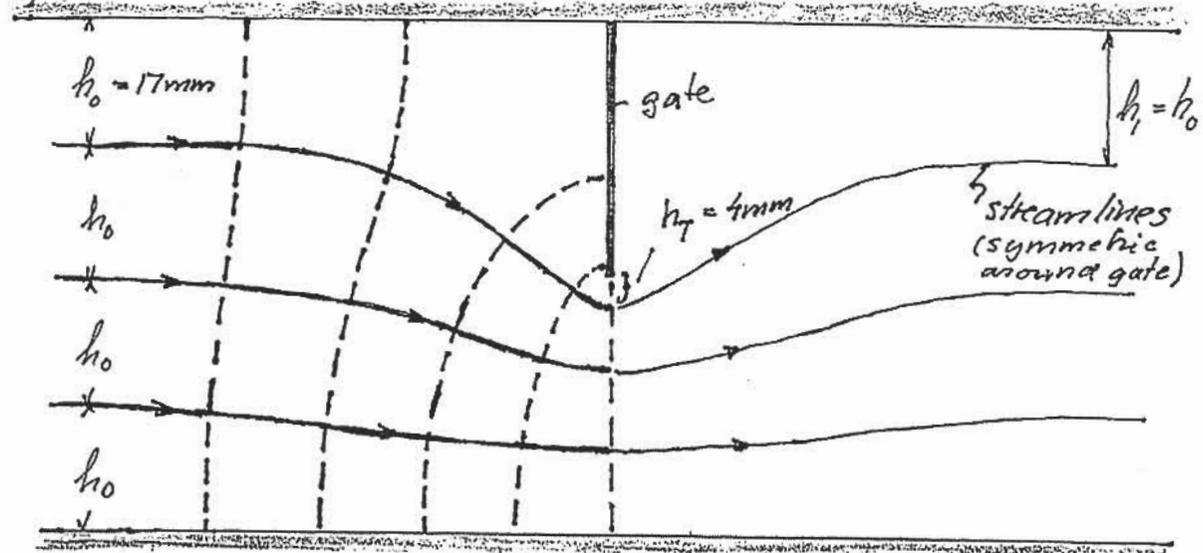
Notice: Flow net is symmetrical with respect to the line along the gate. Streamlines must therefore pass under the gate and be perpendicular to gate's continuation (if they were not, the streamlines would exhibit a sharp corner - a kink - directly below the gate).
