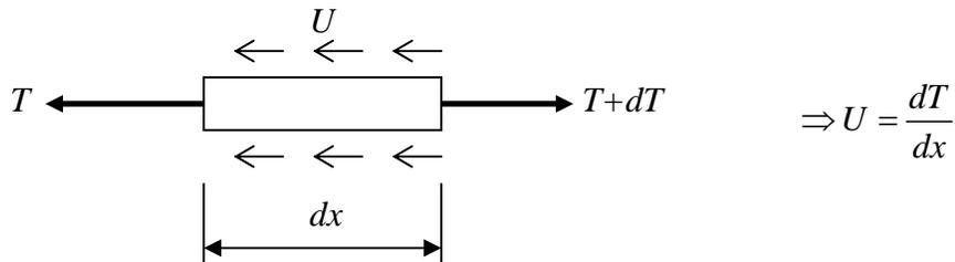
6. Full bond strength needs to be developed to transfer shear forces into the concrete core.
