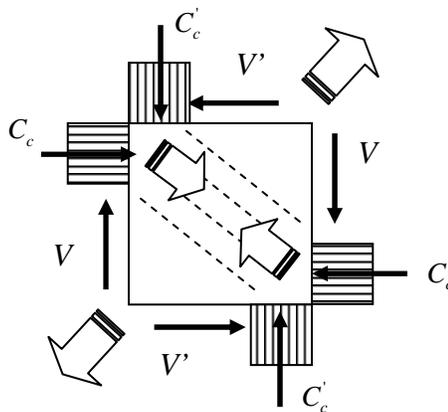
$\rightarrow V_c = C_c - V' =$  shear force transferred through concrete
