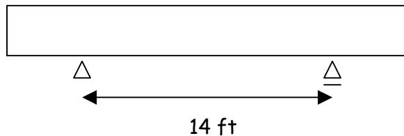
Redesign the shear reinforcement using both approximate and accurate values of  $V_c$  and discuss the effects of changing support configuration for both procedures. Assume  $A_s' = A_s$ .
