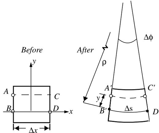
Now  $AC$ , the length of the differential line element in its undeformed state, is the same as the length  $BD$ , namely  $AC = BD = \Delta x = \Delta s$  while its length in the deformed state is  $A'C' = (\rho - y) \cdot \Delta\phi$
