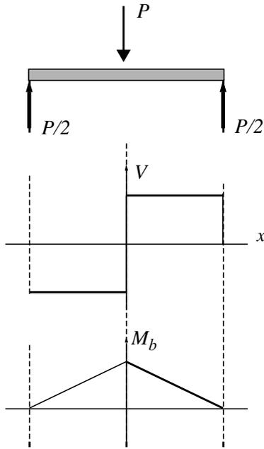
We first sketch the shear force and bending moment diagram, noting that the maximum bending moment occurs at mid span while the maximum shear force occurs at the ends.
