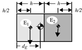
What does this mean? Think of it as a machine for computing the location of the unstrained, neutral axis,  $y = 0$ . However, in this case it is located, not at the centroid of the cross-sectional area, but at the *centroid of area weighted by the elastic moduli*. The meaning of this is best exposed via a short thought experiment. Turn the composite section over on its side. For ease of visualization of the special effect I want to induce I consider a composite cross section
