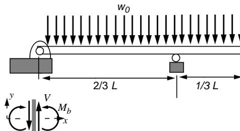
i) Where does the maximum normal stress due to bending occur.
