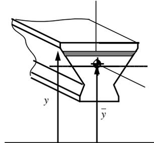
If  $y$  is measured relative to the axis passing through the centroid, then  $\bar{y}$  is zero, our requirement is satisfied.
