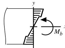
as before, but now, when we replace  $\sigma_x$  with its variation with  $y$  we must distinguish between integrations over the two material, cross-sectional areas. We have then, breaking up the area integrals into  $A_1$  over one material's cross section and  $A_2$ , the other material's cross section<sup>6</sup>
