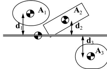
We use the same composite section as above and seek the total moment of inertia of all segments with respect to the centroid of the composite. We first write  $I$  as the sum of the  $I$ 's
