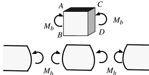
Now run around to the other side of the page and look at the section  $AB$ . The moment looks the same so section  $AB$  too must bulge out. Now come back and consider the portion of the beam to the right of section  $CD$ ; its cross section too would be bulged out. But then we could not put the section back without gaps along the beam. This is an incompatible state of deformation.
