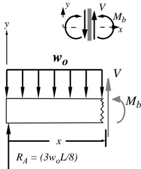
A section of the beam cut between the two supports will enable the evaluation of the shear force and bending moment within this region. We have indicated our positive sign convention as the usual. Force equilibrium gives the shear force
