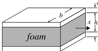
*carries a concentrated load  $P$  at midspan. If the ratio of the thickness of the aluminum face sheets to the thickness of the core is  $t/h = 1/20$  develop an estimate for the maximum shear stress acting at the interface of the two materials.*
