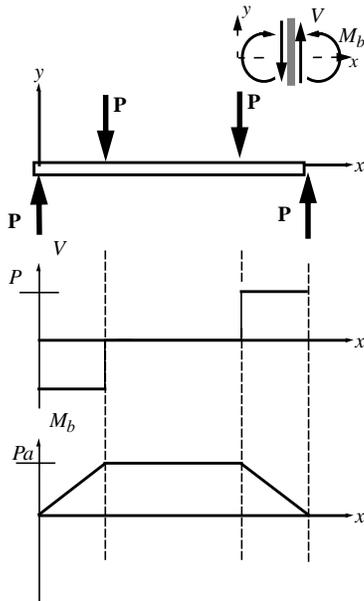
We have already worked up a *pure bending* problem; the *four point bending* of the simply supported beam in an earlier chapter. Over the midspan,  $L/4 < x < 3L/4$ , the bending moment is constant, the shear force is zero, the beam is in pure bending.
