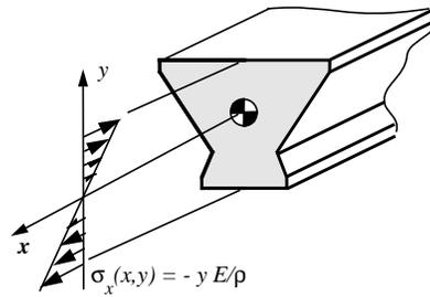
**of the cross section of the beam.** Without this requirement we would be left floating in space, not knowing from whence to measure  $y$ . The centroid of the cross section is indicated on the figure.
