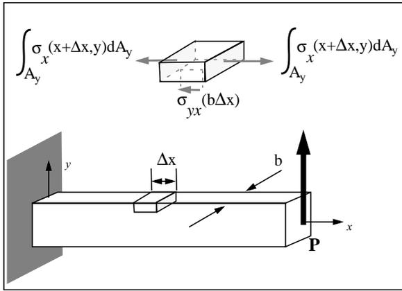
We next develop a more accurate, more detailed, picture of the shear stress distribution making use of an ingenious free-body diagram. Look left.
