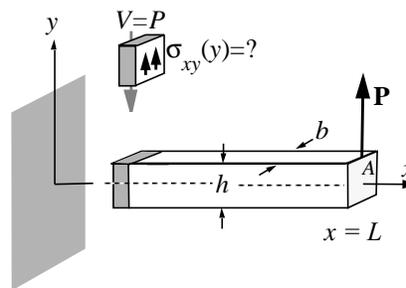
We postulate that this shear force is distributed over the plane cross section at  $x$  in the form of a shear stress  $\sigma_{xy}$ . Of course there is a normal stress  $\sigma_x$  distributed over this section too, with a resultant moment equal to the bending moment at the section. But we do not show that on our picture just yet.
