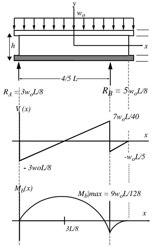
The maximum stress due to this maximum bending moment is obtained from
