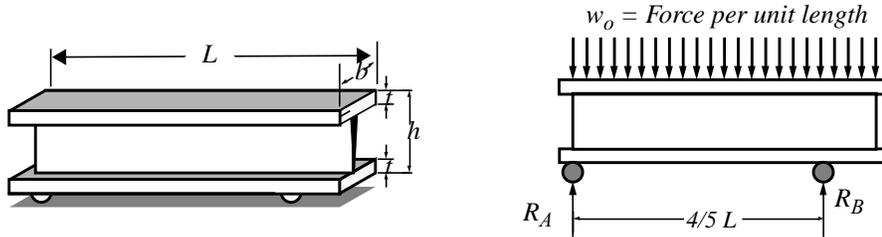
An isolation of the entire span and requiring equilibrium gives the two vertical reactions,
