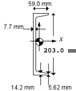
Verify the values given for the mass/length, the cross-sectional area, and the two moments of inertia. (Note that Moment of Inertia (xx) refers to the moment of inertia about the “x-x” axis, what we have labeled, “I”). That is
