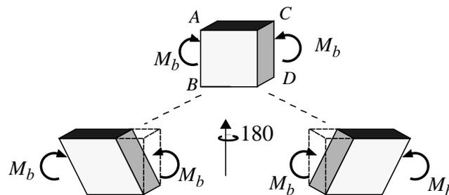
The two alternative deformation patterns shown above are equally plausible – there is no reason why one should occur rather than the other. But rotating either about the vertical axis shown by 180 degrees produces a contradiction. Hence they are both impossible. **Plane cross sections remain perpendicular to the longitudinal axis of the beam.**
