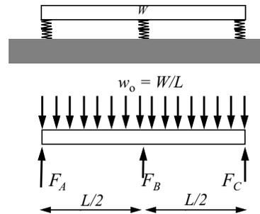
In the same figure, we show a free-body diagram. The forces in the spring, taken as compressive, push up on the beam in reaction to the distributed load. Force equilibrium in the vertical direction gives:
