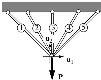
Let's say we have a redundant structure as shown at the left. Now assume we have found all the actual forces,  $f_1, f_2, \dots, f_5$ , in the members by an alternative method yet to be disclosed (it immediately follows this preliminary remark). The actual loading consists of force components  $X_1$  and  $X_2$  applied at the one free node in directions indicated by  $u_1$  and  $u_2$ .
