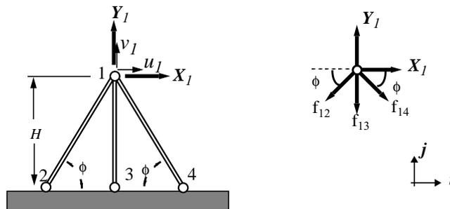
that the equations expressing force equilibrium of node #1 in the  $x$  and  $y$  directions, when phrased in terms of the unknown displacements of the node,  $u_1$ ,  $v_1$ , take the form
