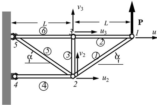
Before proceeding, we review how we might determine the displacements following the path taken in developing the stiffness matrix. We take as an example the statically determinate example of the last section. We simplify the system, applying but one load,  $P$  in the vertical direction at node 1.
