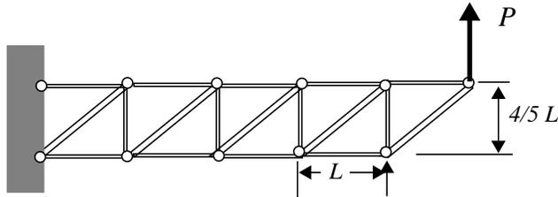
5.7 The truss show below is loaded at midspan with a weight  $P = 60$  lbs. The member lengths and cross sectional areas are given in the figure. The members are all made of steel.
