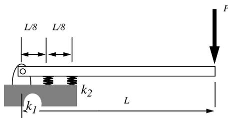
**5.11** The rigid beam is pinned at the left end and supported also by two linear springs as shown.
