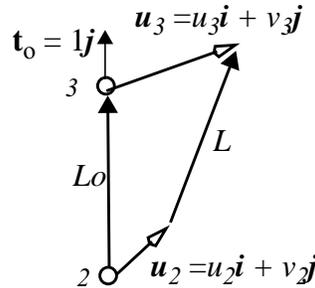
Note how the horizontal displacement components, the  $u$  components, do not enter into this expression for the extension (or compression if  $v_2 > v_3$ ) of member 3. That is, any displacement perpendicular to the member does not contribute to its change its length! This is clearly only approximately true, only true for *small displacements and rotations*.
