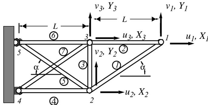
The number of linearly independent equilibrium equations remains the same, namely six, but two of the equations, expressing horizontal and vertical equilibrium of forces at node 3, now include the additional unknown member force  $f_7$ . Leaving to you the task of amending the free-body diagram of node #3, we have
