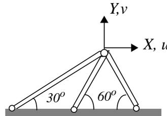
What if a third member, of the same material and cross-sectional area, is added to the structure to stiffen it up; how does the stiffness matrix change?
