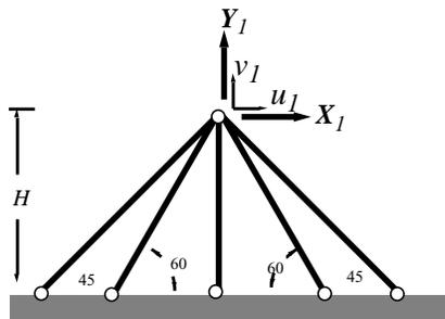
**5.9** For the three problems 1a, 1b, and 1c, state whether the problem posed is statically *determinate* or statically *indeterminate*. In this, assume all information regarding the geometry of the structure is given as well as values for the applied loads.
