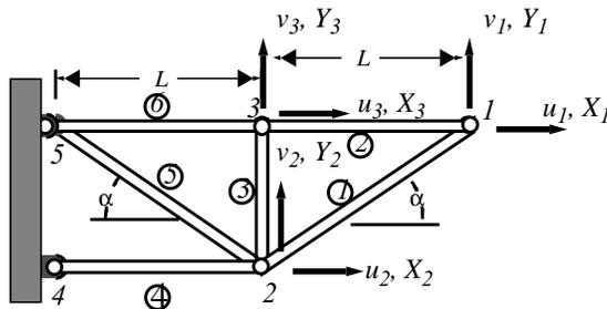
Now consider the truss structure shown above. Although this system is more complex than the previous example in that it has more *degrees of freedom* – six scalar nodal displacements versus two for the simpler truss – the structure is less complex in that it is statically determinate; there are no redundant or unnecessary members; remove any member and the structure would collapse.
