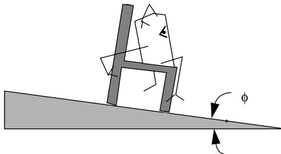
I begin by drawing a free-body diagram, isolating the student and the chair together – all that which will slide down the table top when tipped up – as a particle. The weight  $W$  in the figure below is the weight of the student and the chair. The reaction force at the interface of the chair with the table is represented by two perpendicular components, the normal force  $N$  and the friction force  $F_f$ . We now require that the resultant force on the particle vanish.
