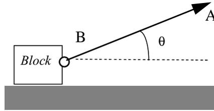
To find the force I must exert, through the cable, onto the block in order to slide it to the right I will isolate the block and apply the laws of static equilibrium. Now this, at first reading, might appear a contradiction: How can the block be sliding to the right and in static equilibrium at the same time?
