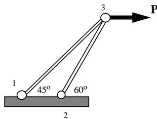
**2.15** Isolate pin 3, showing the forces acting on the pin due to the tension (or compression) in the two members. Find the forces in the members in terms of  $P$ .
