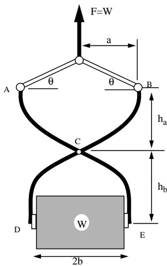
**2.18** The vice grip shown is made of two formed steel members pinned at  $C$ . Construct an expression for the force component which compresses the block at the bottom in terms of the weight of the block  $W$  and the dimensions shown. Express your result in terms of nondimensional factors.
