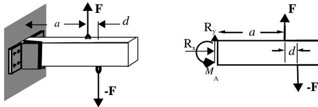
We isolate the cantilever beam, showing all the applied and reaction forces (and couples) acting. This is shown at the right. Note the symbol, the circular arrow. It represents the unknown couple or moment acting at the point A, assumed here to be acting counterclockwise. Force equilibrium requires
