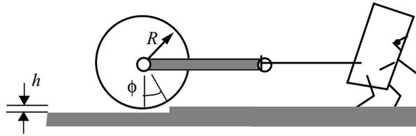
acting upon it. These include the weight acting downward through the center of the roller; the horizontal force applied along the handle by the child laborer (note the frictionless pin fastening the handle to the roller); and the components of the reaction force at the bump, shown as  $N_x$  and  $N_y$ .
