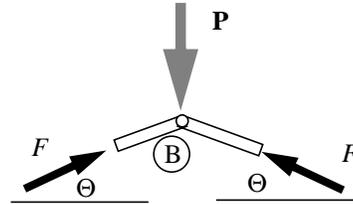
Equilibrium requires that *the resultant force* on the node vanish; symmetry, with respect to a vertical plane containing  $P$  and perpendicular to the page, assures this requirement is satisfied in the horizontal direction; equilibrium in the vertical direction gives:
