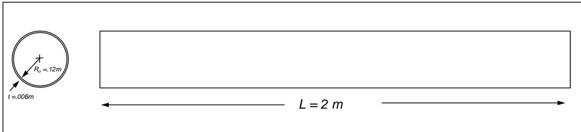
A possible design choice is the point (circled) at  $x = .95$ ,  $y = 0.06$ . This gives an outer radius of  $R_o = 0.12$  m and a wall thickness of  $t = .006$  m.
