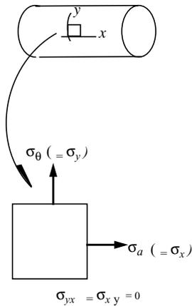
A closed can of soda is under pressure equivalent to that in an automobile tire. We measured the wall thickness in lab on Thursday to be 0.0025 inches. Estimate the axial stress  $\sigma_a$  and the hoop stress  $\sigma_\theta$  acting at a point in this closed, thin cylindrical shell, away from the ends. C
