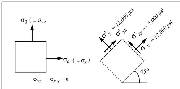
At the left we show the element at the surface of the cylinder before and after rotation of reference axes.
