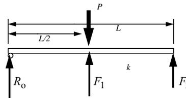
iii) Using the force/deformation relations for the linear springs, express equilibrium in terms of the angle of rotation of the beam.
