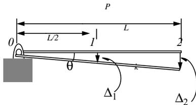
We draw the system in its deflected state. From the geometry, ie. similar triangles, we have, assuming small rotations and displacements
