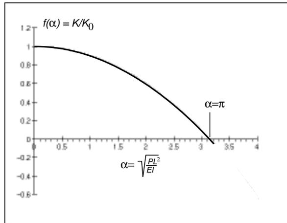
Note that when  $\alpha = \pi$ , the stiffness vanishes! This means that it requires no transverse force  $F$  to produce a transverse displacement! Note too that  $\alpha = \pi$  means that the axial load is just equal to the buckling load of the system found previously.
