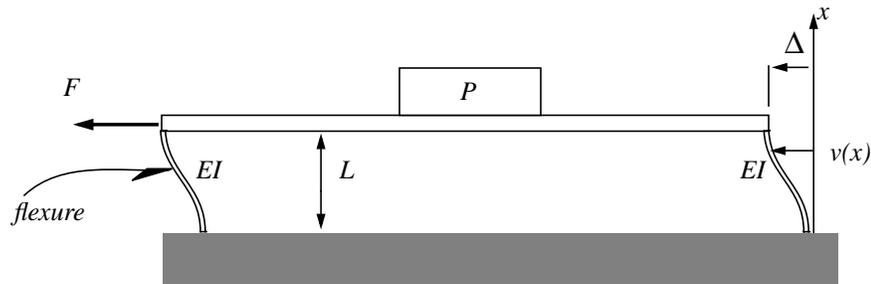
The beam is actually two (or four) identical “flexures” whose ends, firmly fixed to the rigid plate at some distance  $L$  above the “ground” may still move freely in the horizontal direction.
