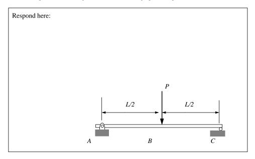
Determine how the internal (bending) moment,  $M_b$ , and internal (shear) force, V, vary with x and P and L.
