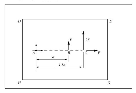
Show, on the redrawn body below, an equivalent system of a i) "couple" and ii) single force vector acting at point A.
