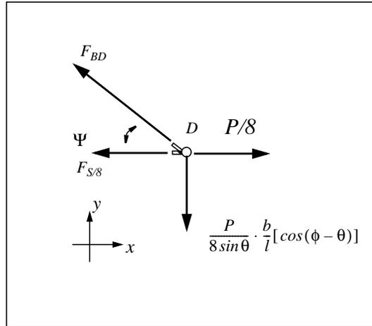
$$\begin{aligned} \sum F_x = 0 & \quad -F_{s/8} - F_{BD} \cdot \cos\Psi + P/8 = 0 \\ \sum F_y = 0 & \quad -\frac{P}{8 \sin\theta} \cdot \frac{b}{l} [\cos(\phi - \theta)] + F_{BD} \cdot \sin\Psi = 0 \end{aligned}$$
