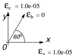
Three strain gages are mounted in the directions shown on the surface of a thin plate. The values of the extensional strain each measures is also shown in the figure.
