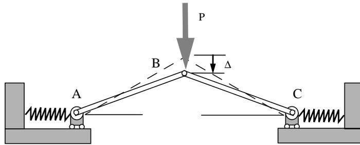
The two-bar linkage is pinned at its ends to linear springs of equal stiffness. The pins A and C are constrained vertically but free to move horizontally. The pin B, where the load is applied, is free to move vertically, even down below the horizontal. (The dashed lines show the unloaded,  $P=0$ , configuration.)
