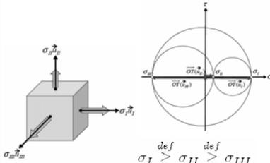
$\sigma_I \stackrel{def}{\geq} \sigma_{II} \stackrel{def}{\geq} \sigma_{III}$ | Principal stresses<br>Principal stress directions<br>Principal stresses and directions obtained through eigenvector analysis<br><i>Principal stresses = Eigenvalues</i><br><i>Principal stress directions = Eigenvectors</i> |
