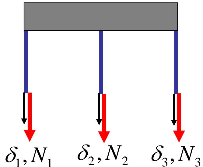
$$\left. \begin{array}{l} N_1 = k\delta_1 \\ N_2 = k\delta_2 \\ N_3 = k\delta_3 \end{array} \right\} \text{Trusses behave like springs}$$
