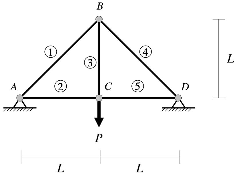
We take advantage of the great tools of energy bounds in elasticity to solve this statically indeterminate truss by applying the *complementary energy approach* to the force-driven problem (recall part 1.3 in Lecture 29, see also slide 11 in the handout for Lecture 29).
