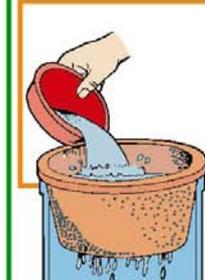
3) Fill the filter several times and discard the filtered water. This will remove the taste of the clay.
