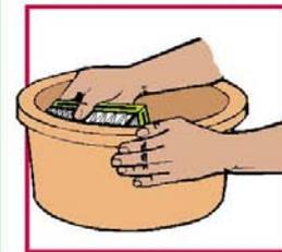
2) Using water from the receptacle, fill the filter half way and scrub it vigorously with a brush to unclog the pores. Discard the dirty water. You will have some small particles of clay come off if you are scrubbing hard enough.
