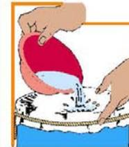
4) If your river or well water is cloudy, use a piece of cloth over the filter element to prefilter the water each time. Tie a string around the cloth so that it does not fall into the filter.
