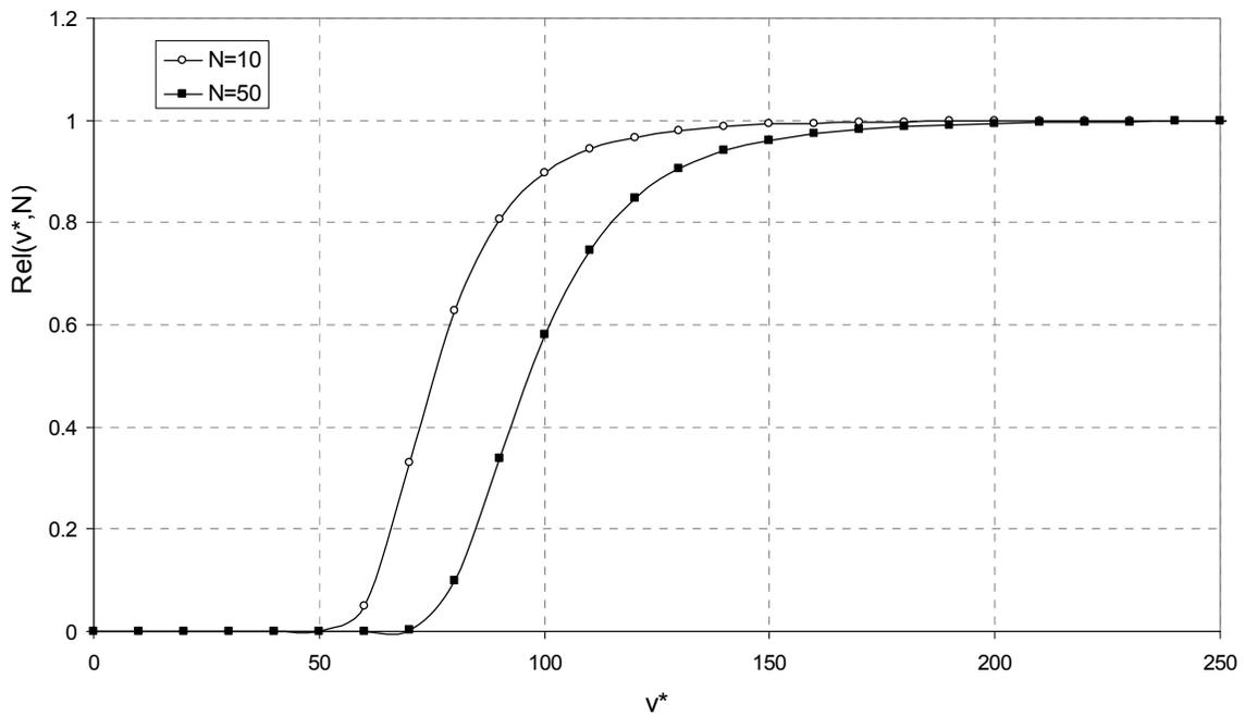
**Figure 1: Reliability of a building in Boston against wind as a function of design wind speed  $v^*$ , for exposure periods of 10 and 50 years.**
