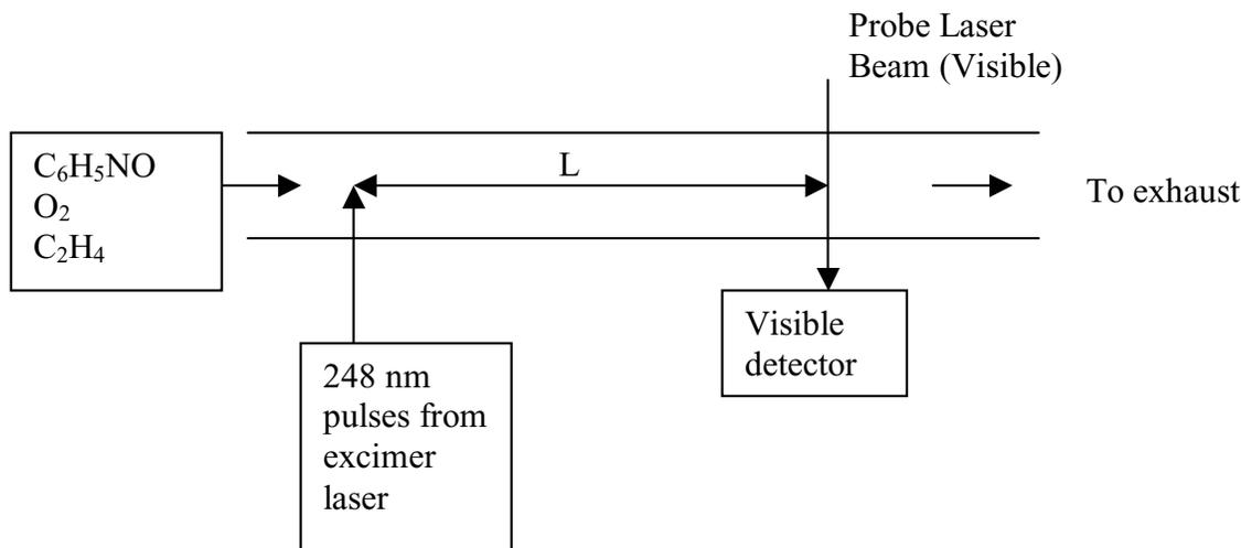
The experimental adjustables are flow distance  $L$ , the mass flow rates of each of the 3 input gases, the diameter of the tube  $d$ , the temperature  $T$ , and the pressure  $P$ . The measurable is the Intensity of visible laser light measured by the detector. The excimer is firing at a steady rate of 50 pulses per second and its average power of 5 W appears to be constant over the course of the experiment. The incident intensity of the visible (probe) laser beam is also constant in time.
