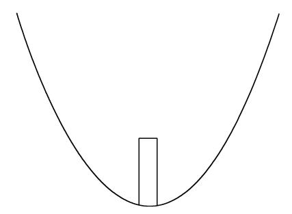
For a thin barrier, all  $\psi_v$  with node in middle (odd v) hardly feel barrier. They are shifted to higher E only very slightly.
