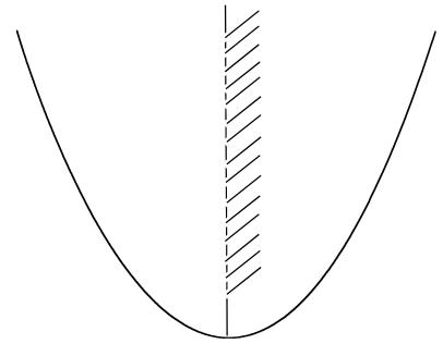
This half-HO oscillator only has levels at  $E_1$ ,  $E_3$  of the full oscillator so v = 0 of ½ oscillator is at the energy of v = 1 of the full oscillator.
