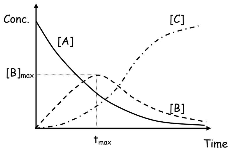
$$t_{\max}^B = \frac{\ln(k_1/k_2)}{k_1 - k_2} \quad \text{with } k_1 \neq k_2 \quad [B]_{\max} = \frac{k_1}{k_2} [A]_0 e^{-k_1 t_{\max}^B}$$
