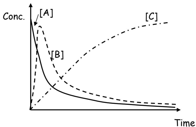
$B \xrightarrow{k_2} C$  is the rate determining step
