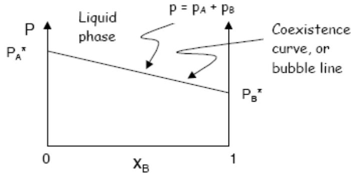
The gas phase is described by  $y_A$  or  $y_B$ . If  $T$  and  $x_A$  are given, then  $y_A$  and  $y_B$  are fixed (by Gibbs phase rule). That is, if  $T$  and the composition of the liquid phase are known, then the composition of the gas phase is determined.
