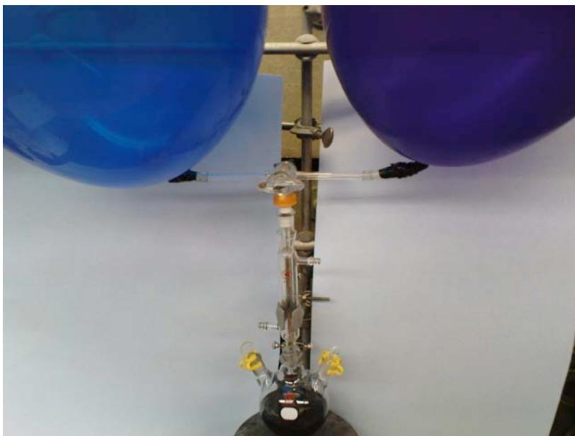
**Figure 2. Hydrogenolysis reaction setup.**
