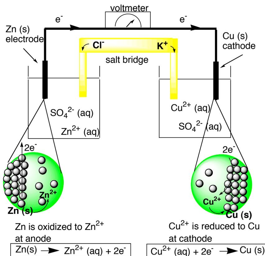
Anode (Oxidation) Electrons produced from oxidation flow out of compartment through a wire. Positive charge increases in the compartment due to the production of  $Zn^{2+}$  from  $Zn^0$ . To maintain neutrality,  $Cl^-$  flows in through the salt bridge.
