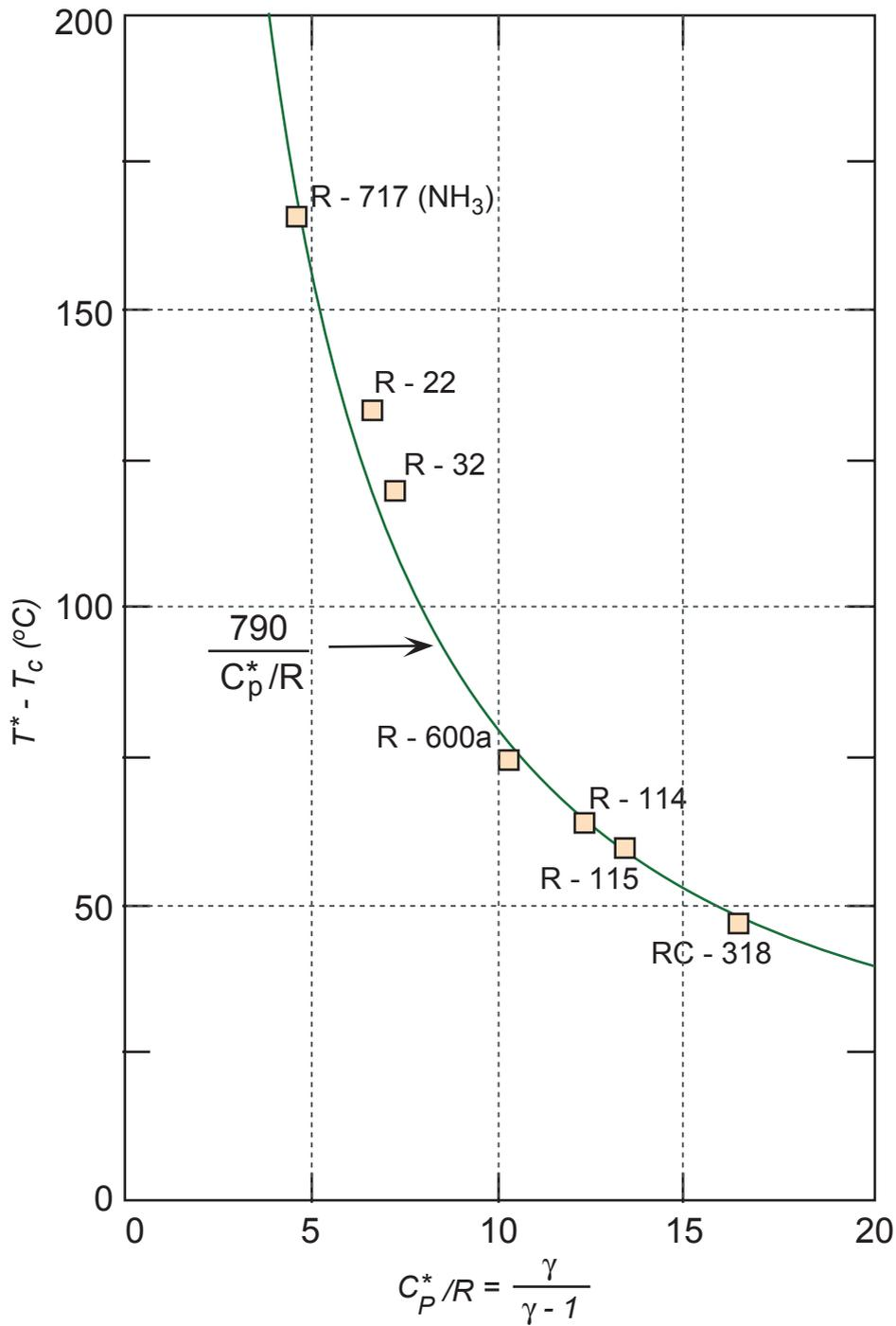
Generalized correlation for the degree of superheat above the critical temperature for optimum utilization of geothermal fluid availability as a function of ideal gas state reduced heat capacity.
