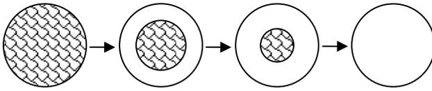
**Figure 7.** Shrinking core model
