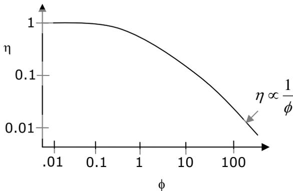
**Figure 6.** Log-log plot of effectiveness factor versus thiele modulus
