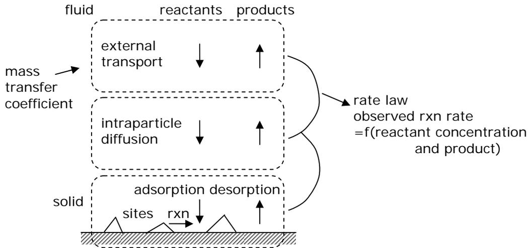
**Figure 1.** Schematic of surface reaction kinetics.
