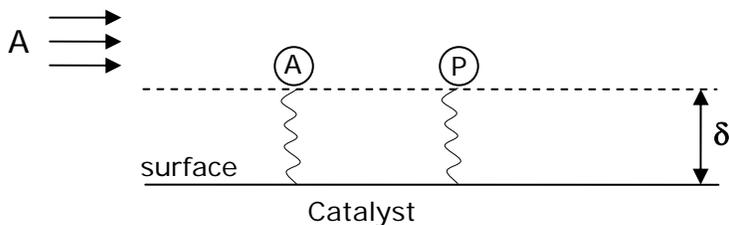
**Figure 1.** Schematic of boundary layer at catalyst surface for a turbulent, well mixed system where  $C_A$  is a function of  $x$ .
