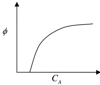
**Figure 9.** Fractional yield versus concentration when  $\alpha_1 > \alpha_2$ .
