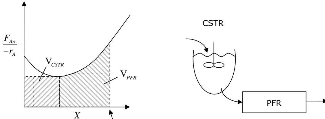
**Figure 7.** To achieve the desired conversion with smaller reactor volumes, use a combination. In this case, use a CSTR then a PFR. By doing so, the reactor volume is less than the area underneath the curve.
