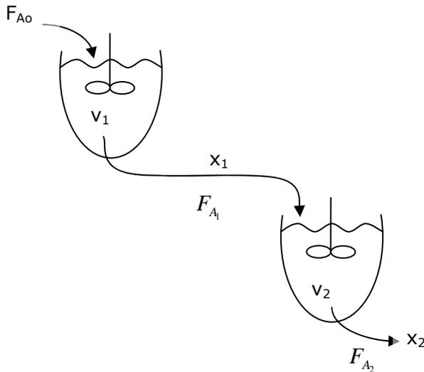
**Figure 3.** Schematic of two CSTRs in series.
