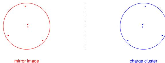
Figure 2: Electrostatic system: two well-separated, symmetric clusters of charges.
