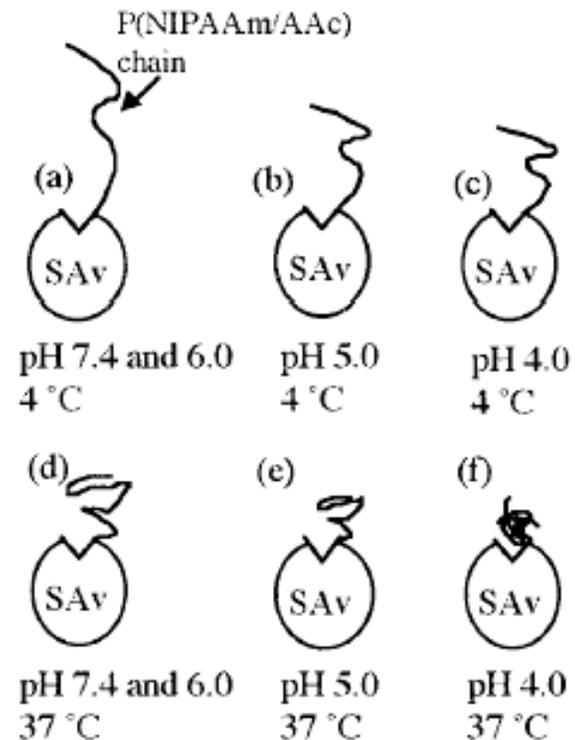
**Figure 6.** Proposed conformations of the polymer chain coils of poly(NIPAAm-co-AAc) conjugated to mutant streptavidin (SAv) at various pHs at 4 and 37 °C.
