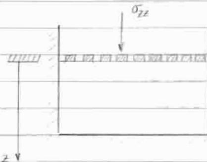
Poroelastic stress relaxation response under confined compression conditions; when a "sinusoidal steady state" displacement  $u(z=0, t) = u_0 \cos \omega t$  is applied.
