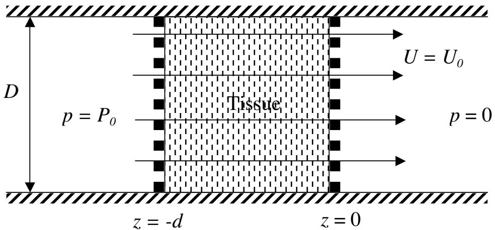
A cylindrical disk of porous, hydrated tissue has thickness  $d$  and diameter  $D$ , and is held within a chamber that confines the disk at its radial periphery. the tissue is supported by a rigid, porous filter located at the position  $z = 0$ . A constant pressure drop  $P_0$  is applied across the tissue from left to right, resulting in a constant fluid flow velocity  $U_0$  with respect to the tissue (the rigid filter prevents the tissue from moving, but does not impeded fluid flow).
